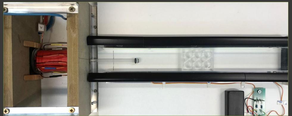
Figure 2. Hand-crafted « coilgun » inertia-driven model used to accelerate the 6-well module to 12.5 m/s reproducing an acceleration/deceleration injury. The module is in plexiglass to reduce friction forces as well as to reduce weight. Coilgun is made of a copper coil crossed by a 220V current previously loaded in 6 capacitors. The strong current crossing the coil generates a powerful magnetic field pushing the piston which accelerates the module on the track.
